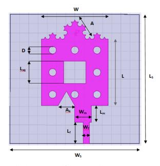
Fig. 4. Geometry of the proposed antenna.
